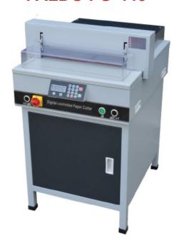
Faldo FO-455 paper cutter for office use. Digital controlled paper cutter with transparent safety cover on the front and metal cover on the back with cabinet. Automatic clamping and automatic cutting. Back gauge digital controlled by keypad. Main switch and safety lock, electronically controlled, two-hand operation. Blade depth adjustment from outside of the machine. Optical cutting line. Standard with HSS blade. Comes standard including cabinet.
